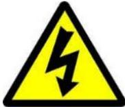
Symbol with lightning flash with arrowhead, within an equilateral triangle is intended to alert the user to the presence of uninsulated dangerous voltage inside the product that may be of sufficient magnitude to constitute a risk of electric shock.
